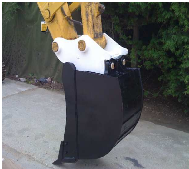
Gravity locking plates which are both always in the locked position unless the bucket is specifically positioned to be removed.
